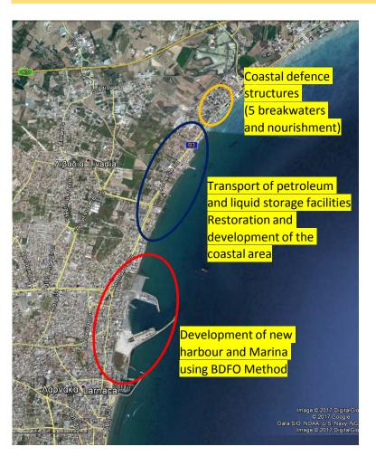
First phase realization: the Ministerial Public Works Department started (Nov 2016) the construction of 5 detached breakwaters in combination with nourishment in the area next to storage facilities (2,2 M€) – June 2018
